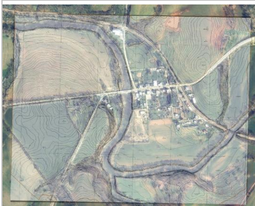
A color aerial photo under a semi-transparent topographic map
